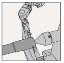
7. Calibrate the MAPAL MASTERSET using a setting gauge (must be ordered separately). The setting gauge is the smallest dimension of the bore.
