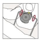
4. Note: Two wrenches must be used for tightening. Press the indexable insert firmly into the indexable insert seat. To tighten the clamping plate turn the TORX® screw or the threaded spindle clockwise from above and counter-clockwise from underneath and tighten.
