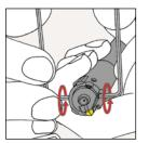
Note: Two wrenches must be used for undoing. To release the clamping plate turn the TORX<sup>®</sup> screw or the threaded spindle counter-clockwise from above and clockwise from underneath.
