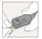
Remove the indexable insert. Clean the insert and the indexable insert seat (do not use compressed air, pay attention to adjusting wedge).
