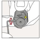
For coarse setting, turn again the threaded pin one quarter of a turn clockwise.
