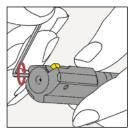
1. Turn the front and rear threaded pin half a turn counter-clockwise.
