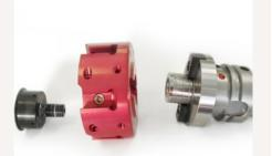
1. Clean the mounting area of the tool and the hydraulic clamping arbor using a cloth.
