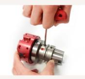
3. Note: The centring screws is not secured against falling out.
