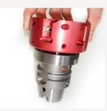
2. Place the tool, with bore and face connection first, on the face connection of the hydraulic clamping arbor.
