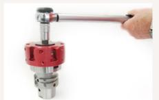
4. Set the torque wrench to the tightening torque of 7 Nm. Tighten the milling cutter clamping screw to the stop with the aid of the torque wrench. Mount the tool in accordance with the information from the manufacturer or using the milling cutter clamping screw in accordance with DIN 6367.
