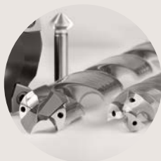
Drilling from the solid, boring and countersinking
