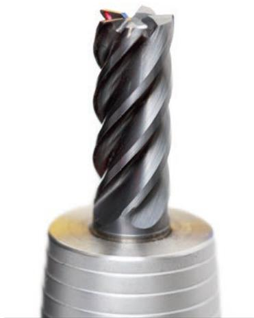
Detail view of a solid carbide end milling cutter with projected laser spot for rough alignment of the measuring position.
