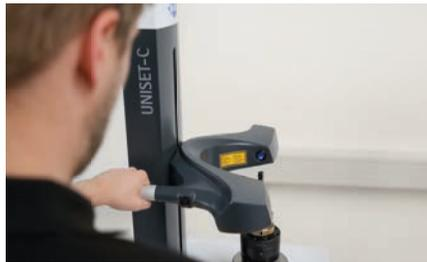
**1** After the milling cutter has been clamped in the tool spindle on the UNISET-C, the measuring arm is moved roughly to the cutting edge. This task can be undertaken very quickly with the aid of the laser. The cutting edge on the milling cutter is then positioned at the cross hair on the monitor with the aid of the fine adjusting wheel.
