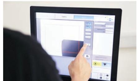
**2** To measure the length and width of the cutting edge, the buttons "X" and "Z" are selected on the monitor. After actuation, the measurement is undertaken immediately and automatically and the measurement results are displayed on the monitor.
