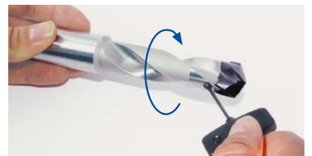
3. Tighten the clamping screw by turning it clockwise tight by hand.
