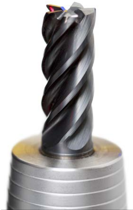
Detail view of a solid carbide end milling cutter with projected laser spot for rough alignment of the measuring position.
