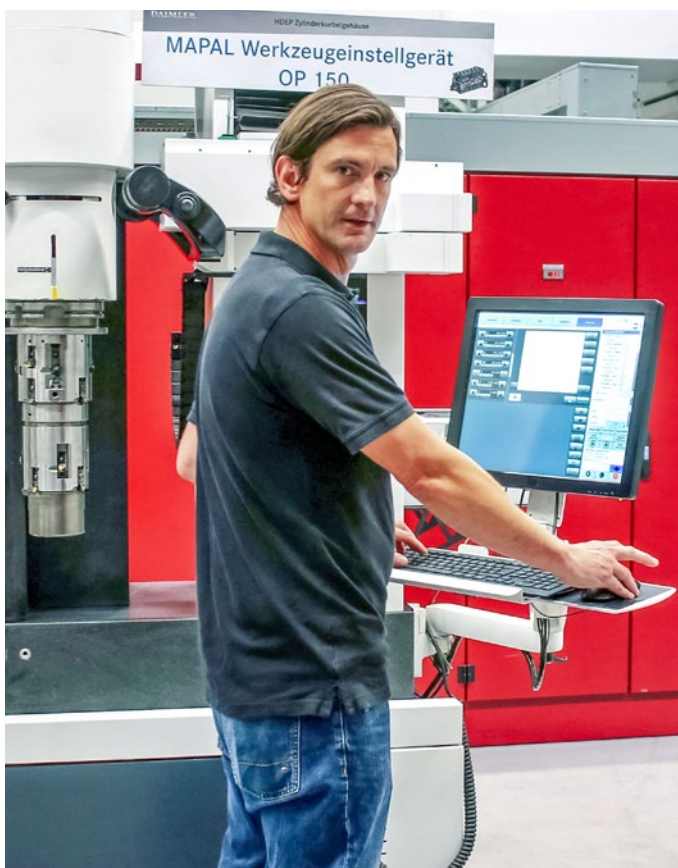
MAPAL application engineer Christoph Wilhelm works on the measuring and setting fixture with a hanging tool arrangement developed specially for this application.
