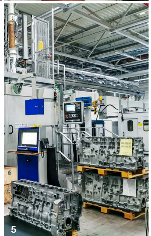
3 Three bores are machined simultaneously with three spindles. A sister tool is stored in the machine for each tool.
