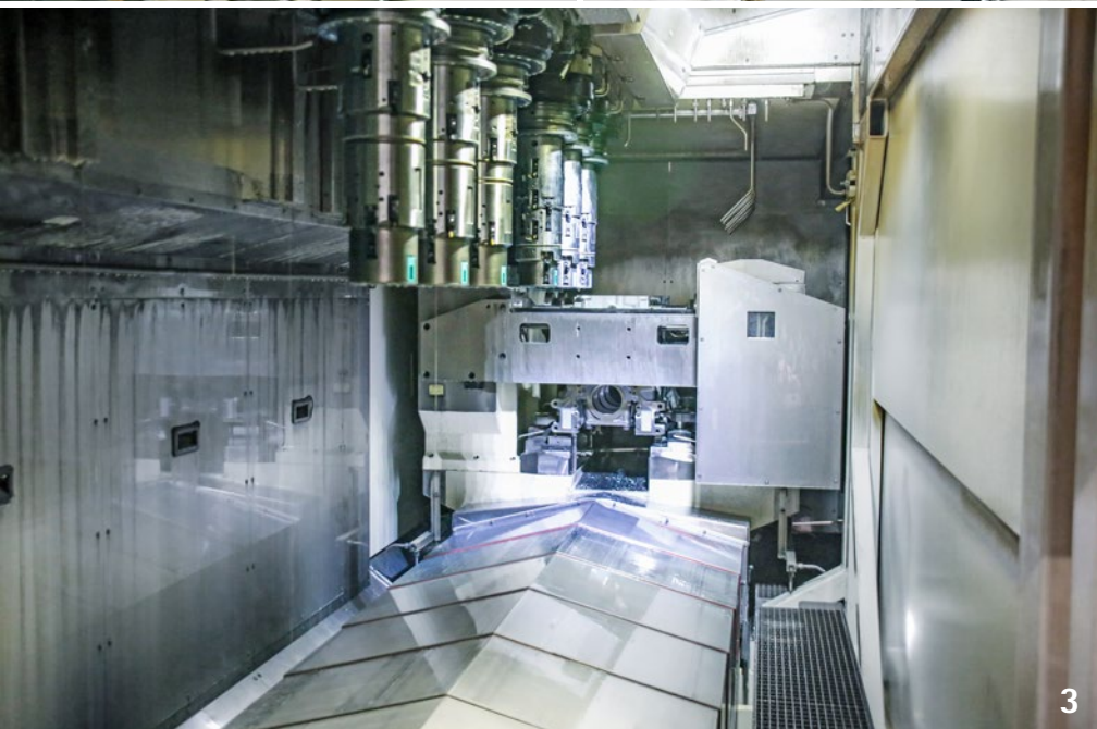
3 Three bores are machined simultaneously with three spindles. A sister tool is stored in the machine for each tool.
