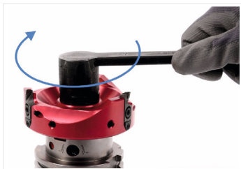
Fig. 7: Tighten the milling cutter clamping screw
