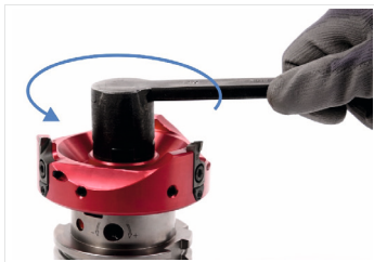
Fig. 8: Loosening the milling cutter clamping screw
