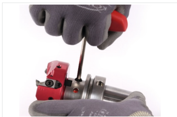
Fig. 9: Loosening clamping screw
