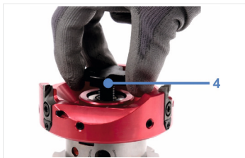
Fig. 5: Screwing in the milling cutter clamping screw
