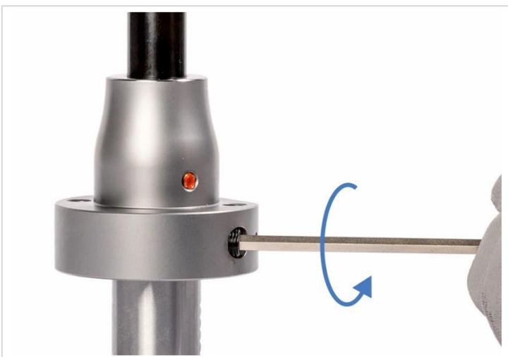
Fig. 17: Loosening clamping screw
