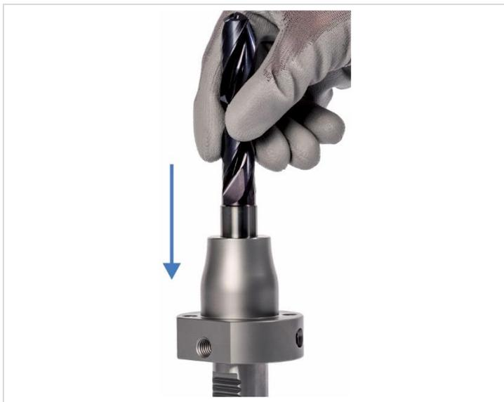
Fig. 10: Inserting tool
