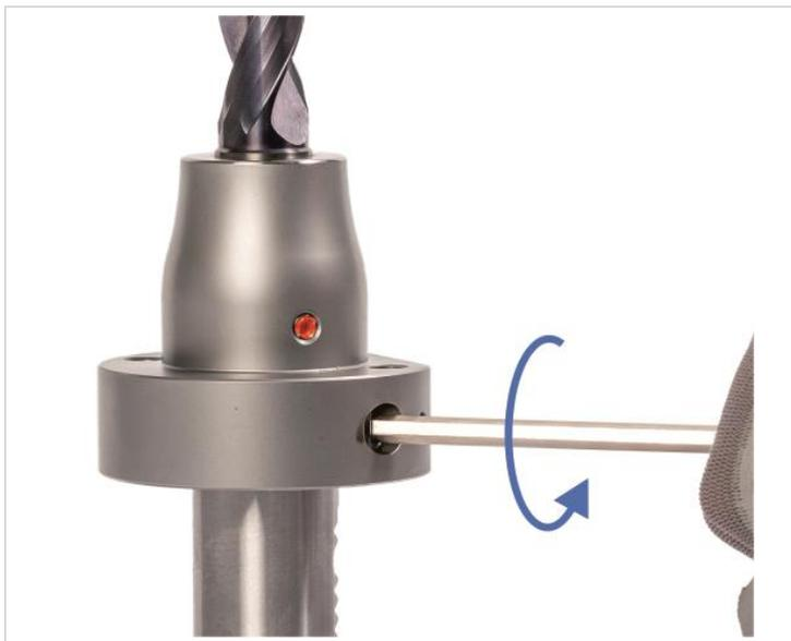
Fig. 12: Loosening clamping screw
