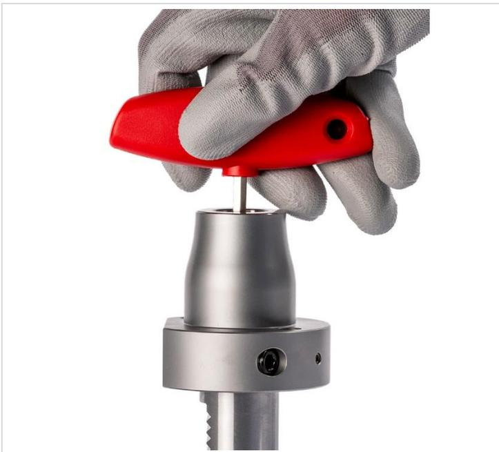
Fig. 8: Adjusting tool length (axial)
