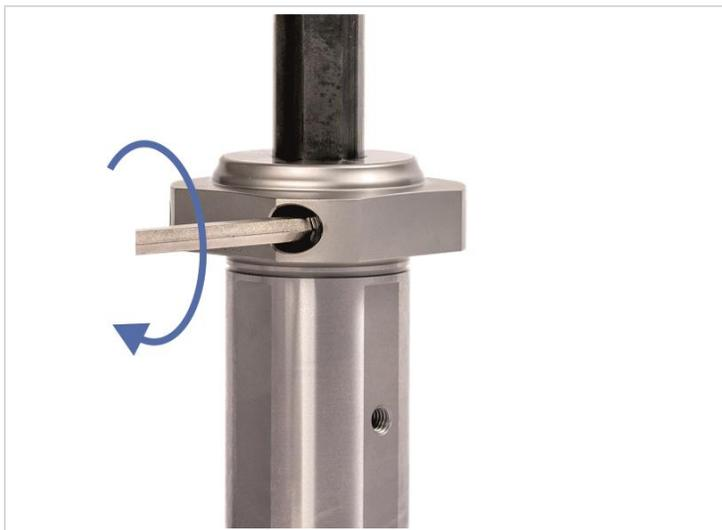
Fig. 21: Tightening clamping screw
