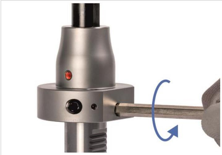
2. Loosen the locking screw using an appropriate hex-wrench with T-handle.
