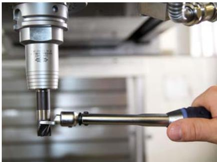
4. Place the torque wrench on the replaceable milling head so it is as horizontal as possible; do not tilt the faces of the spanner.
