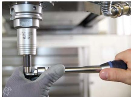
5. **Note:** Place your free hand on the replaceable milling head to be able to adjust it sensitively. In this way the tightening torque can be set more accurately.
