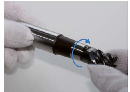
3. Screw the replaceable milling head clockwise into the replaceable head holder so it is hand-tight. Then clamp the replaceable head holder with the tool in the machine holder.
