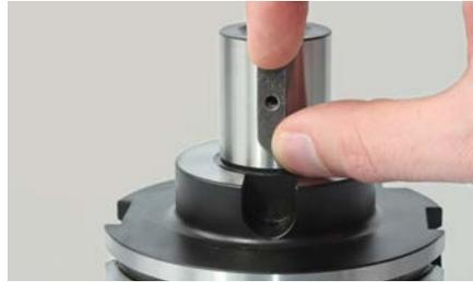
2. Fit the parallel key to the milling cutter arbor.
