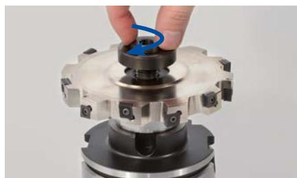
7. Lightly screw the milling cutter clamping screw clockwise into the milling cutter arbor.
