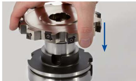
5. Fit the tool flat on the milling cutter arbor.
