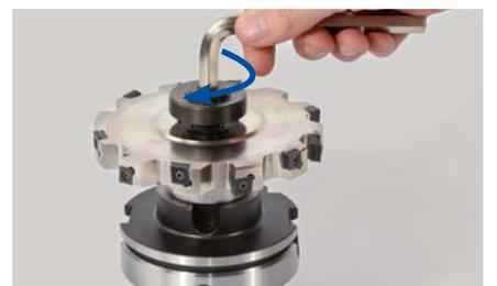
8. Continue to screw the milling cutter clamping screw clockwise with the aid of a hex-wrench and then tighten using a torque wrench (for tightening torque see table "Tightening torque for milling cutter clamping screw").
