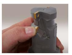
**3.** Press the cassette and the adjusting wedge forward in the direction of the tool.
