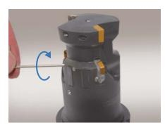
**1.** Loosen the adjusting wedge using a hex-wrench and turn it half a turn counter-clockwise.
