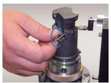
**9.** Set the radial distance or absolute dimension for the indexable insert, for this purpose turn the threaded pin clockwise using a hex-wrench.
