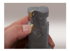
**5.** Replace or turn the indexable insert. Then fit the indexable insert in the cassette.
