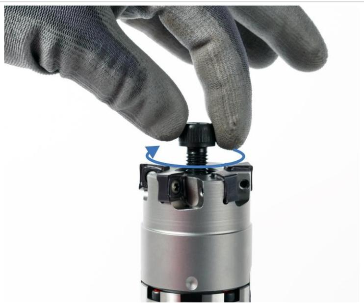
4. Screw the milling cutter clamping screw into the threaded bore of the milling cutter arbor slightly by hand.
