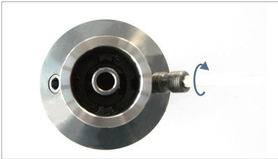
Figure 10: Tightening the gripper screw onto the connection contour on the machine spindle
