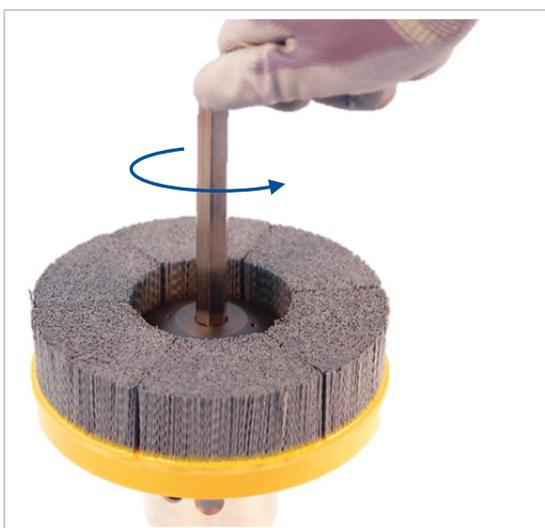
Figure 7: Loosening and removing clamping screw
