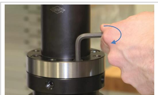
Figure 5: Tighten the axial fastening screws to about **2 Nm**
