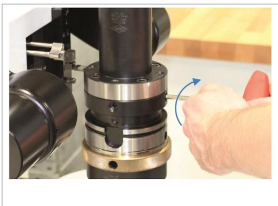
Figure 10: Turning the radial adjusting screws
