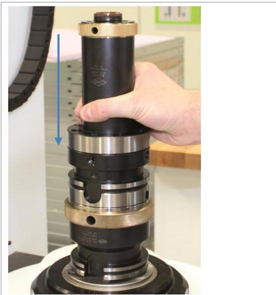
Figure 4: Inserting the KS flange adapter
