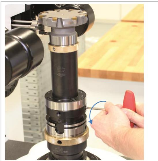
Figure 8: Releasing the radial adjusting screws
