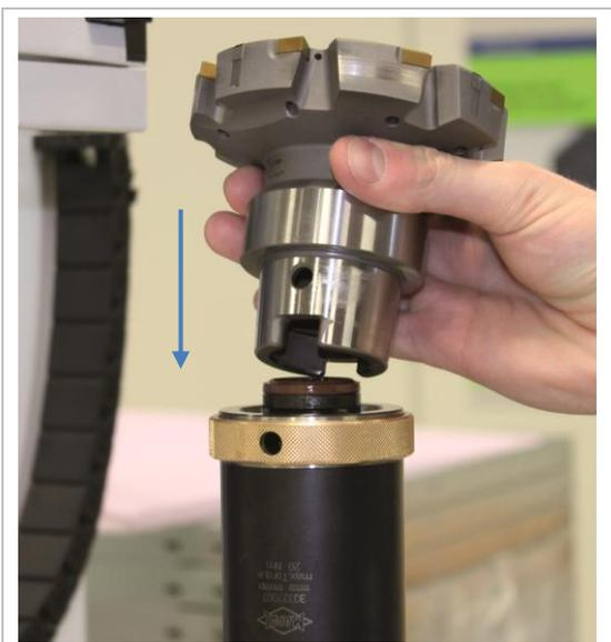
Figure 6: Inserting the TFB fine boring head
