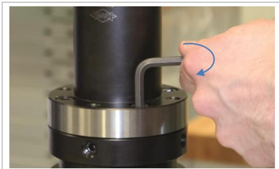
Figure 15: Tightening the axial fastening screws exactly
