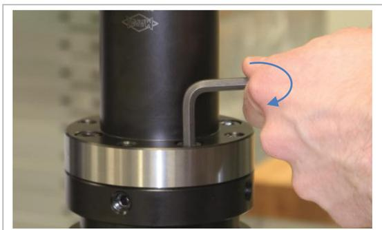
Figure 11: Tightening the axial fastening screws to 50%
