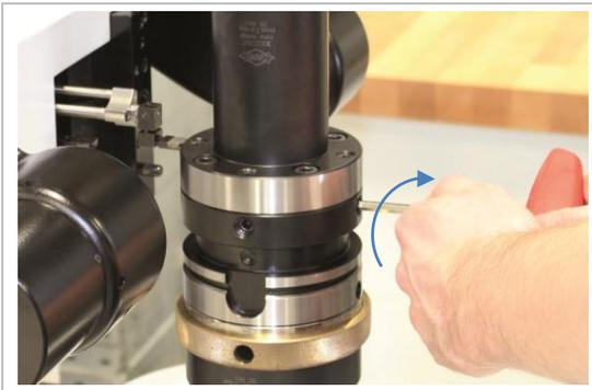
Figure 13: Turning the radial adjusting screws precisely
